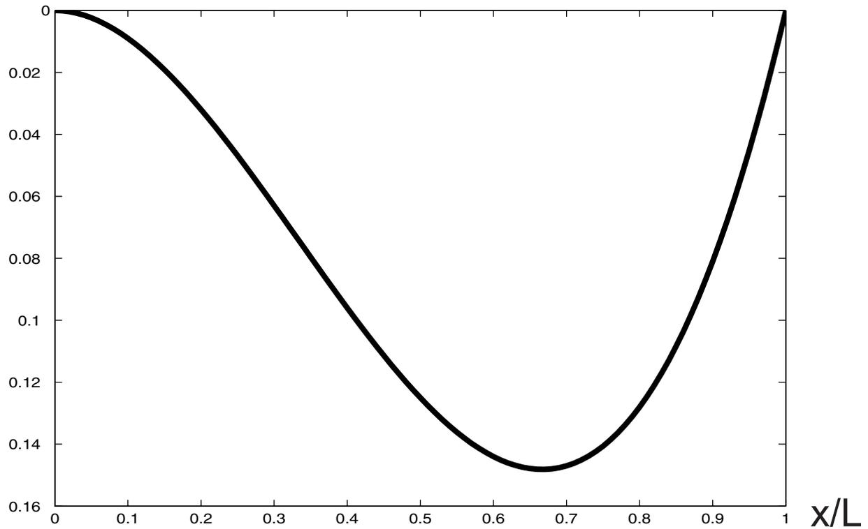
$$v_{total} = \frac{1}{2} K_{(thermal)} x^2 + \frac{R_{tip} x^2 (3L - x)}{6EI} = \frac{\alpha \Delta T^* L^2}{2h} \left( \frac{x}{L} \right)^2 \left( \frac{x}{L} - 1 \right)$$
