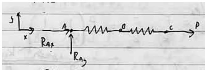
$$\begin{aligned}\sum F_x &= 0 \\ R_{Ax} + P &= 0 \\ R_{Ax} &= -P\end{aligned}$$
