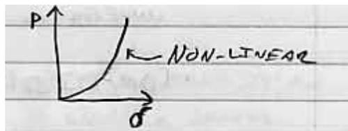
Elastic: Loading and unloading are along the same curve.
