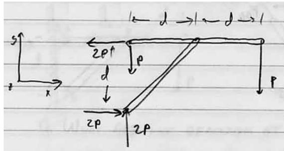
*Statically Determinate:* A situation in which the equations of equilibrium determine the forces and moments that support the structure.
