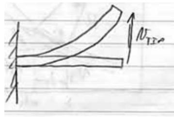
$$\text{So, } v_{tip} = \frac{ML}{2EI}, \theta_{tip} = \frac{ML}{EI}.$$
