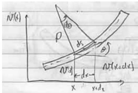
$$ds = \rho d\theta \Rightarrow d\theta = \frac{1}{\rho} ds, \theta = \frac{dv}{dx}, \frac{d\theta}{dx} = \frac{d^2 v}{dx^2} \Rightarrow d\theta = \frac{d^2 v}{dx^2} dx$$
