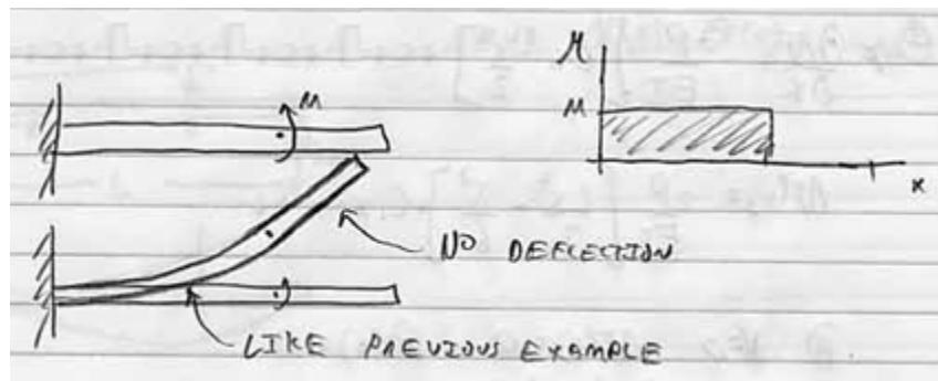
EX: End loaded cantilever beam
