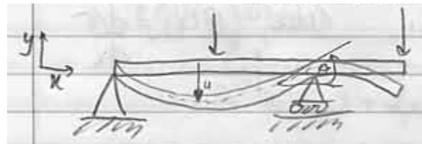
$u(x)$  - Beam deflection,  $\theta(x)$  - beam slope,  $\theta(x) = \frac{dv(x)}{dx}$
