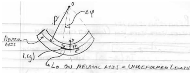
$L_0$  on neutral axis = Undeformed Length
