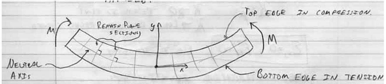
If it is in compression on one side and tension on the other, there must be a plain with no strain. This is called the neutral axis.
