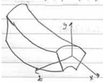
$\epsilon_{yy}$  extends the height of the compressed side and shrinks the height of the tensile side.
