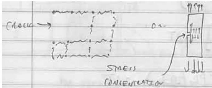
Brittle failure will occur at a stress concentration (defect). This stress concentration will decay within a couple times the size of the defect.
