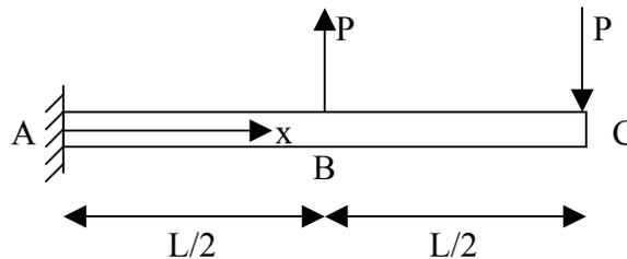
**Problem 4:** Using superposition, calculate the deflection in the center (point B) of the beam shown below. The beam has a moment of inertia  $I$  and a Young's modulus  $E$ .
