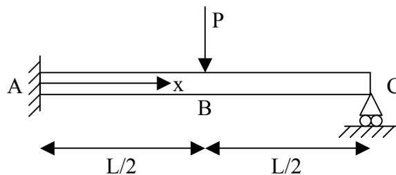
**Problem 5:** Calculate the deflection at the tip of the cantilever below. The half near the support has a Young's modulus of  $E_1$ , and the half away from the support has a Young's modulus of  $E_2$ . The moment of inertia of the beam is  $I$  all the way along its length. You are welcome to use the table in Appendix C whenever it would be useful.
