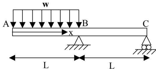
**Problem 3:** Calculate the deflection and slope at the center of the beam below using superposition and the results in Appendix C.
