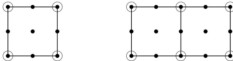
Figure 6.16:  $Q_2$  velocities  $\bullet$  and  $Q_1$  pressures  $\circ$ : failure on one square, success on two.
