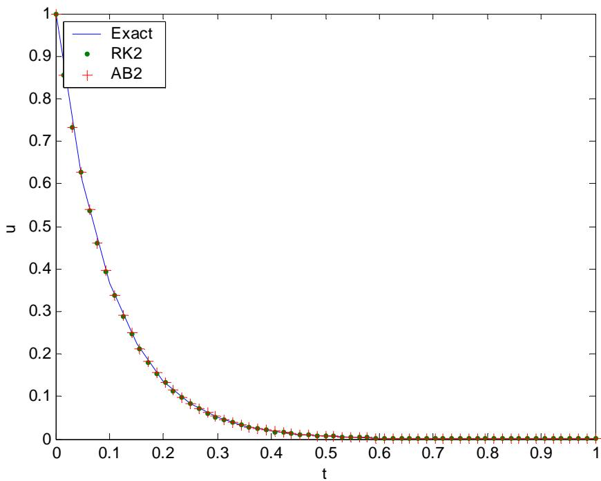
2) Accuracy test (set initial h=0.1 in “HW1\_2.m”)
