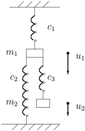
(b) What 3 by 2 matrix  $A$  gives the spring stretching  $e = Au$  from the displacements  $u_1, u_2$  of the masses?
