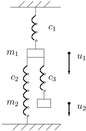
(b) What 3 by 2 matrix  $A$  gives the spring stretching  $e = Au$  from the displacements  $u_1, u_2$  of the masses?
