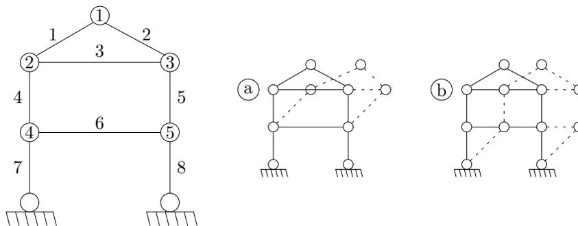
8 bars, 7 nodes, 4 fixed displacements ( $u_6^H, u_6^V, u_7^H, u_7^V$ ). So  $n = 2(7) - 4 = 10$ , and  $10 - 8 = 2$  solutions.
