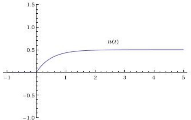
Figure 2: The unit impulse response  $w(t)$  for  $D^2 + 2D$ .
