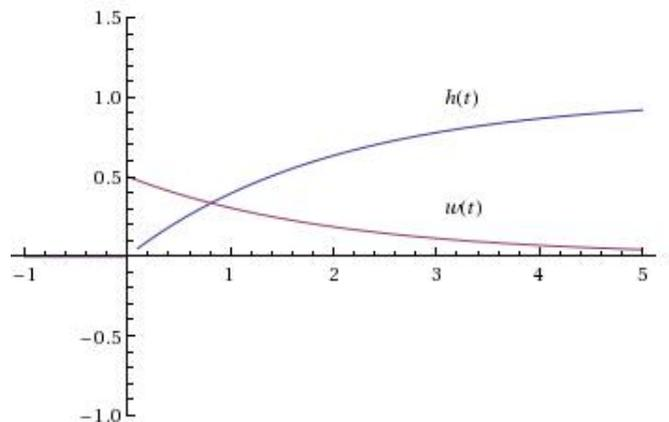
Figure 1: The unit step response  $h(t)$  and unit impulse response  $w(t)$  for  $2D + I$ .
