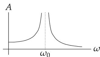
Undamped amplitude response
