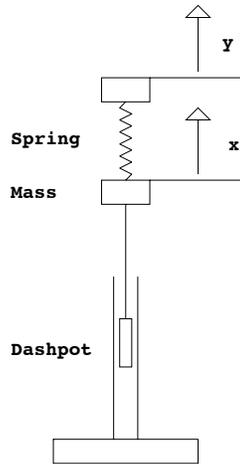
Figure 1. Spring-driven system
