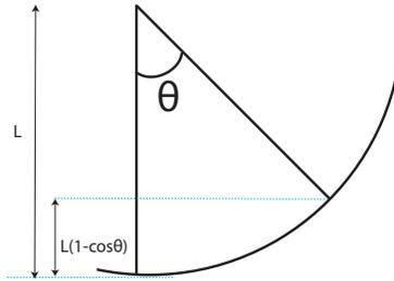
Figure 3: Effect of gravity on a pendulum.
