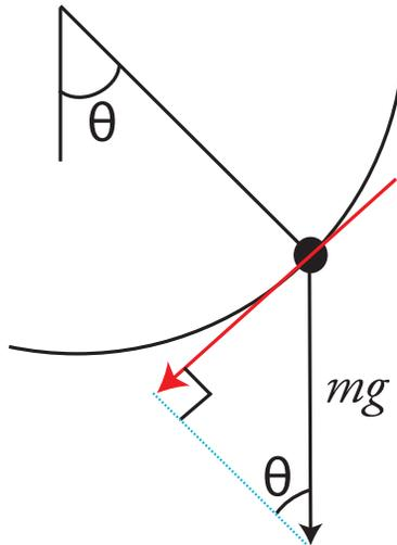
Figure 2:  $F = mg \sin \theta$  (force tangent to path of motion).
