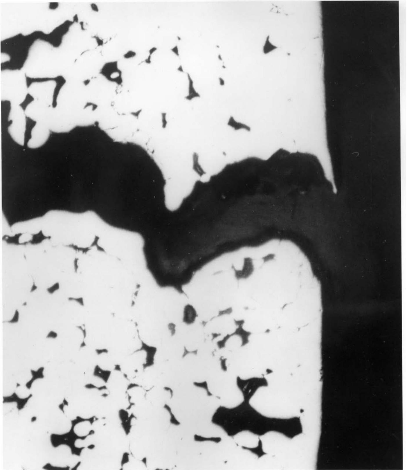
Figure 3: As-polished fractured gutter support casting. (200X)
