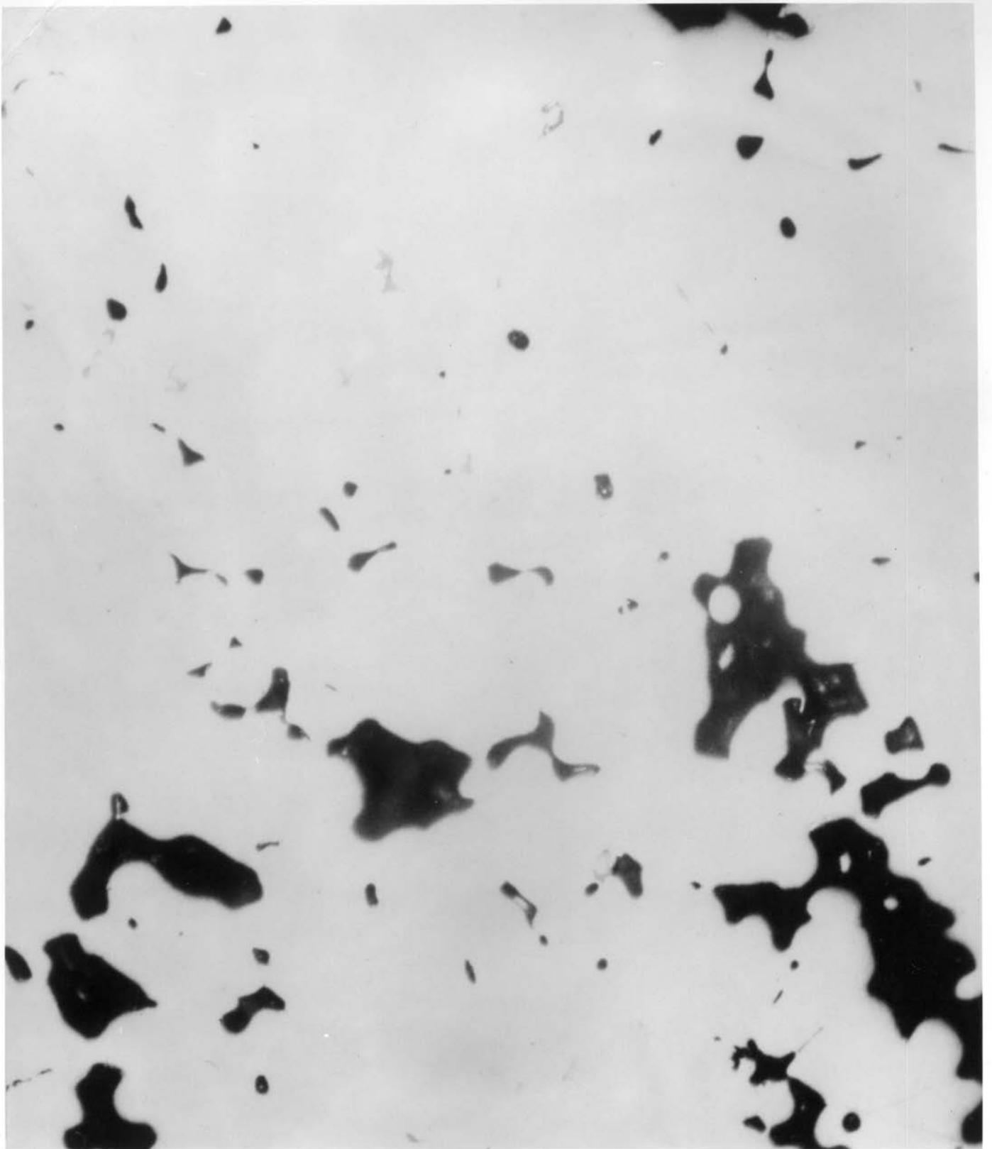
Figure 8: As-polished interior of fractured primary casting. (200X)
