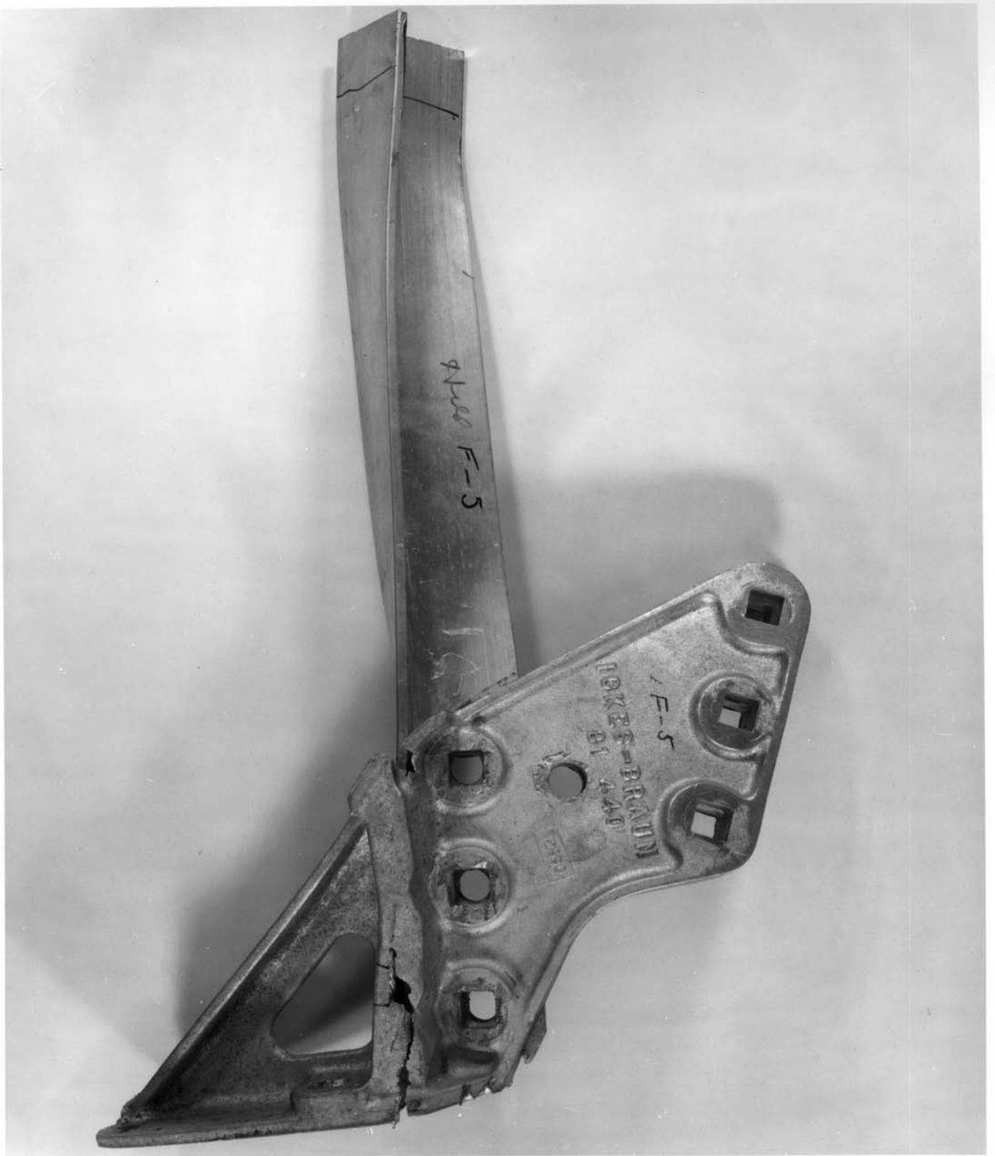
Figure 5: Fractured primary casting with roof chord.
