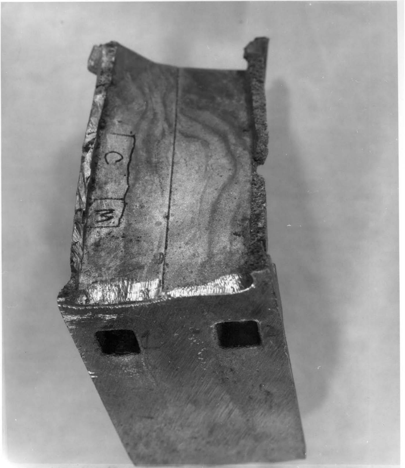
Figure 10: Another fractured primary casting.
