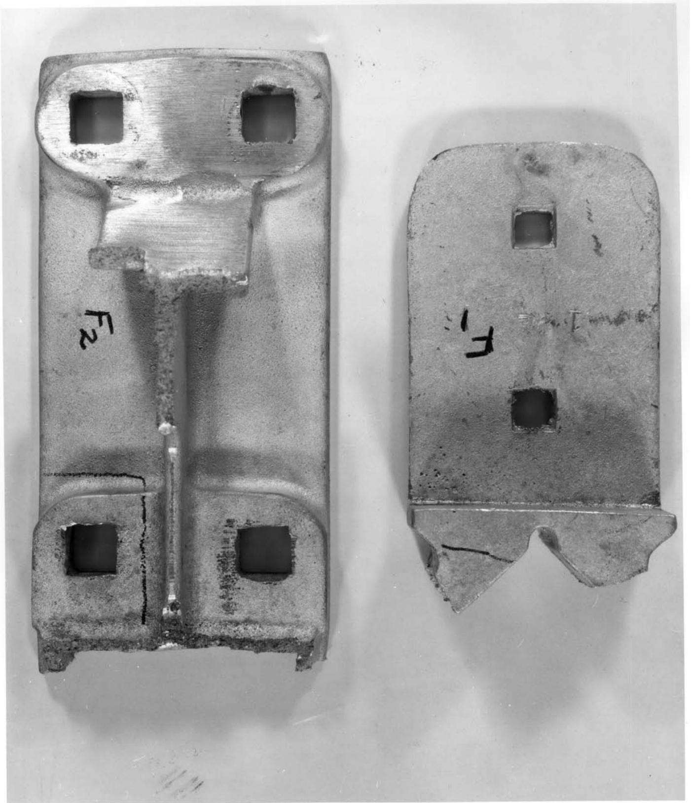
Figure 1: Fractured gutter support casting (right).
