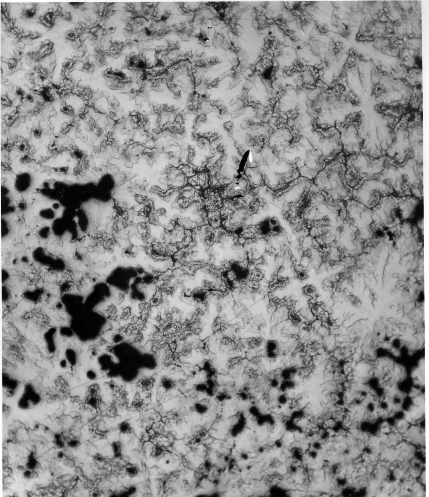
Figure 9: Etched interior of fractured primary casting. (100X)
