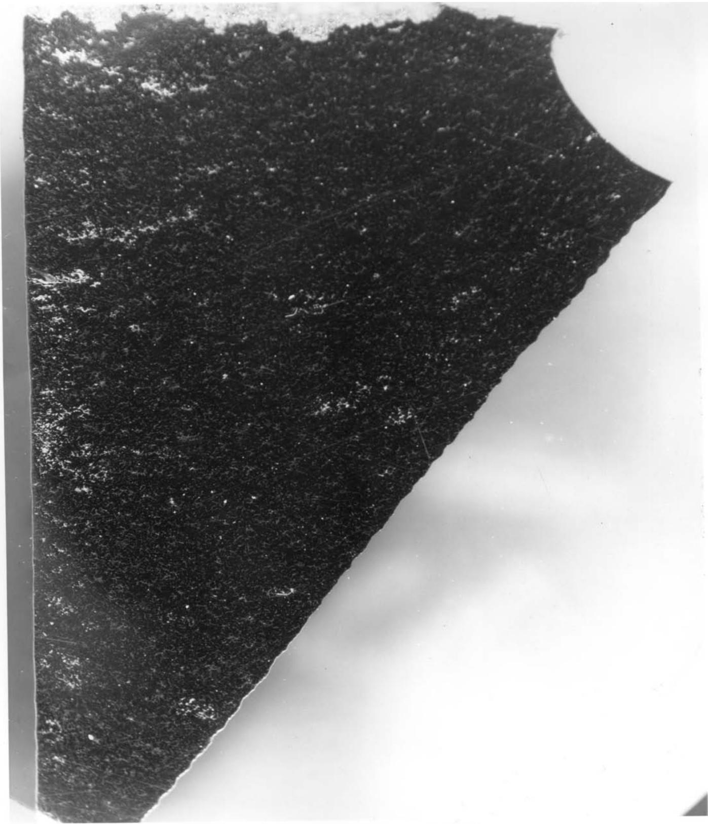
Figure 2: Photomicrograph of fractured gutter support.
