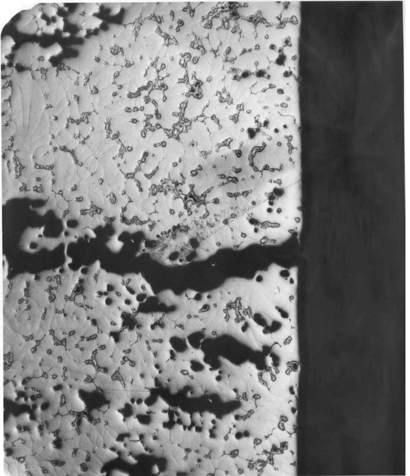
Figure 4: Etched fractured gutter support casting. (100X)
