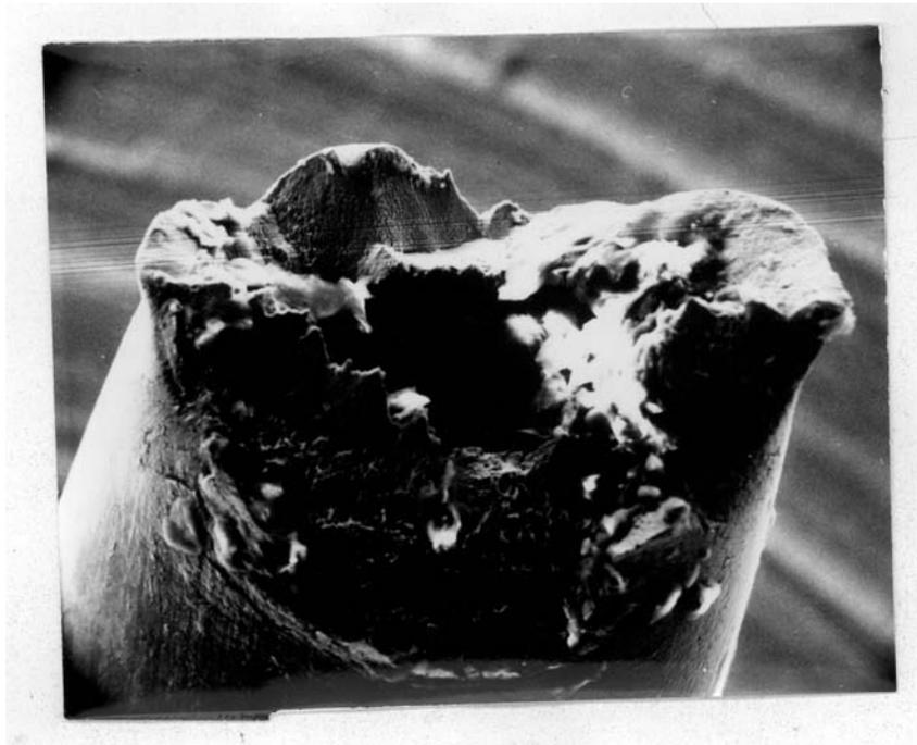
Figure 2: S.E.M. picture of fracture on extra needle. (260X)
