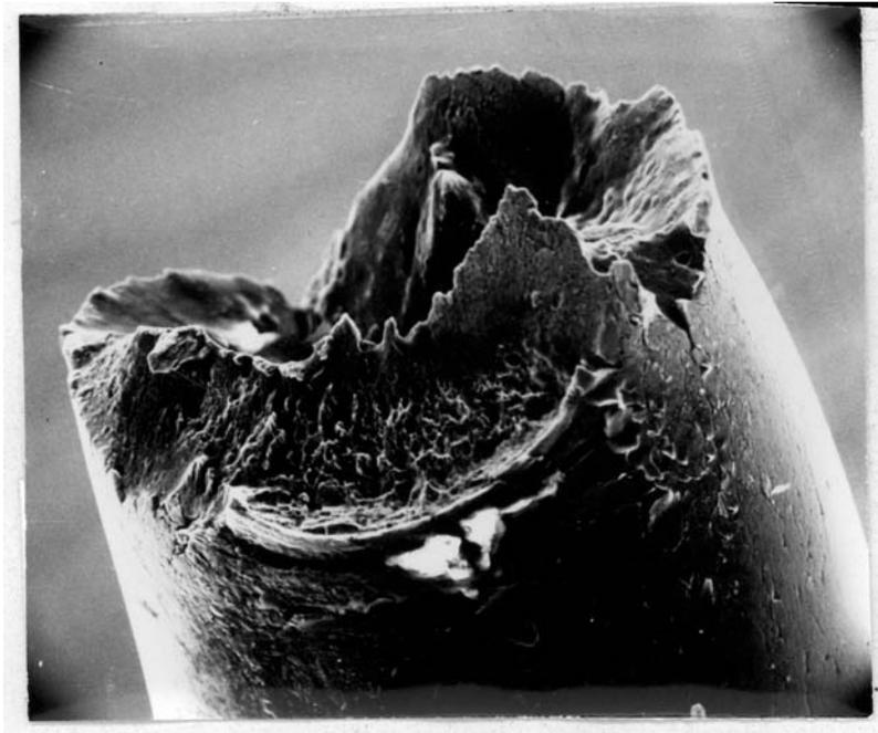
Figure 6: S.E.M. picture of fracture surface in subject needle. (280X)
