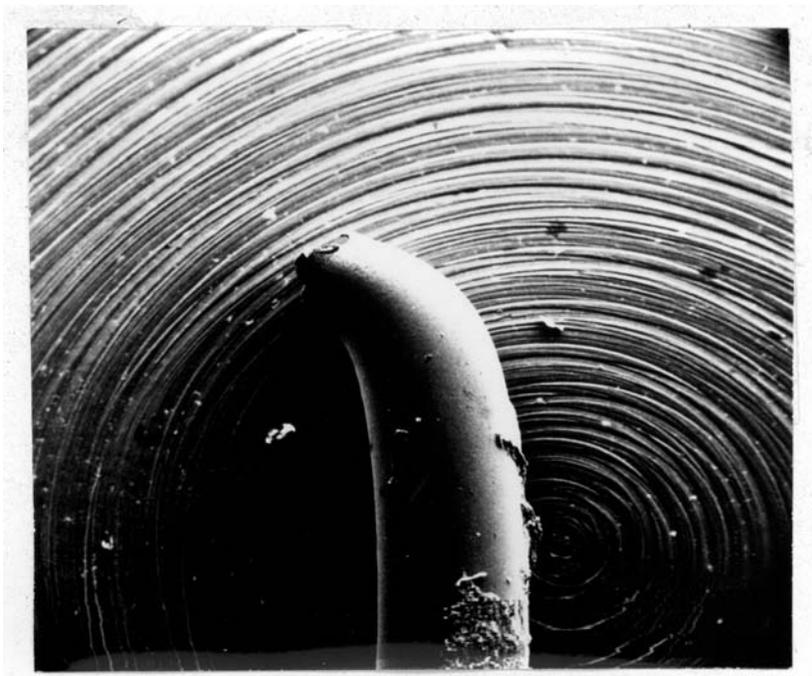
Figure 5: Plan view of needle showing bending that occurred before fracture. (64X)
