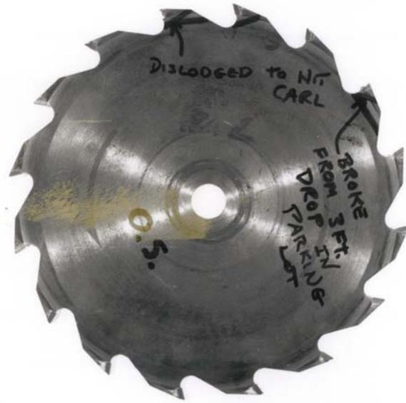
Figure 2: Subject blade, showing multiple broken teeth.
