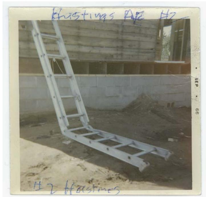
Figure 2: Failed aluminum ladder.
