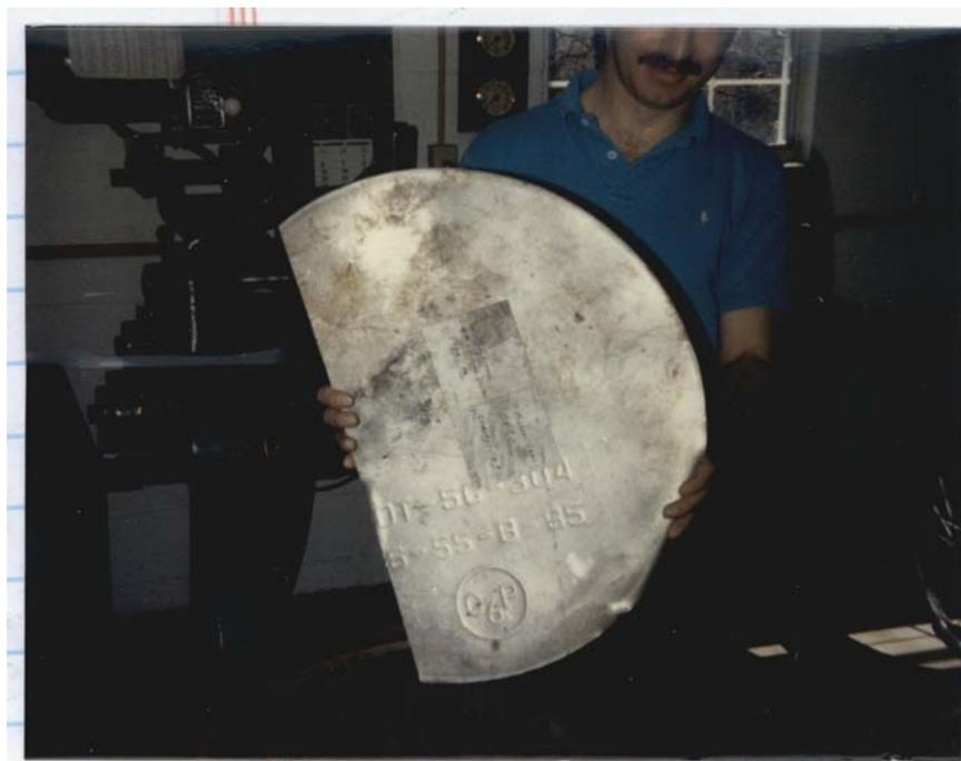
Figure 3: Corroded lid of barrel.
