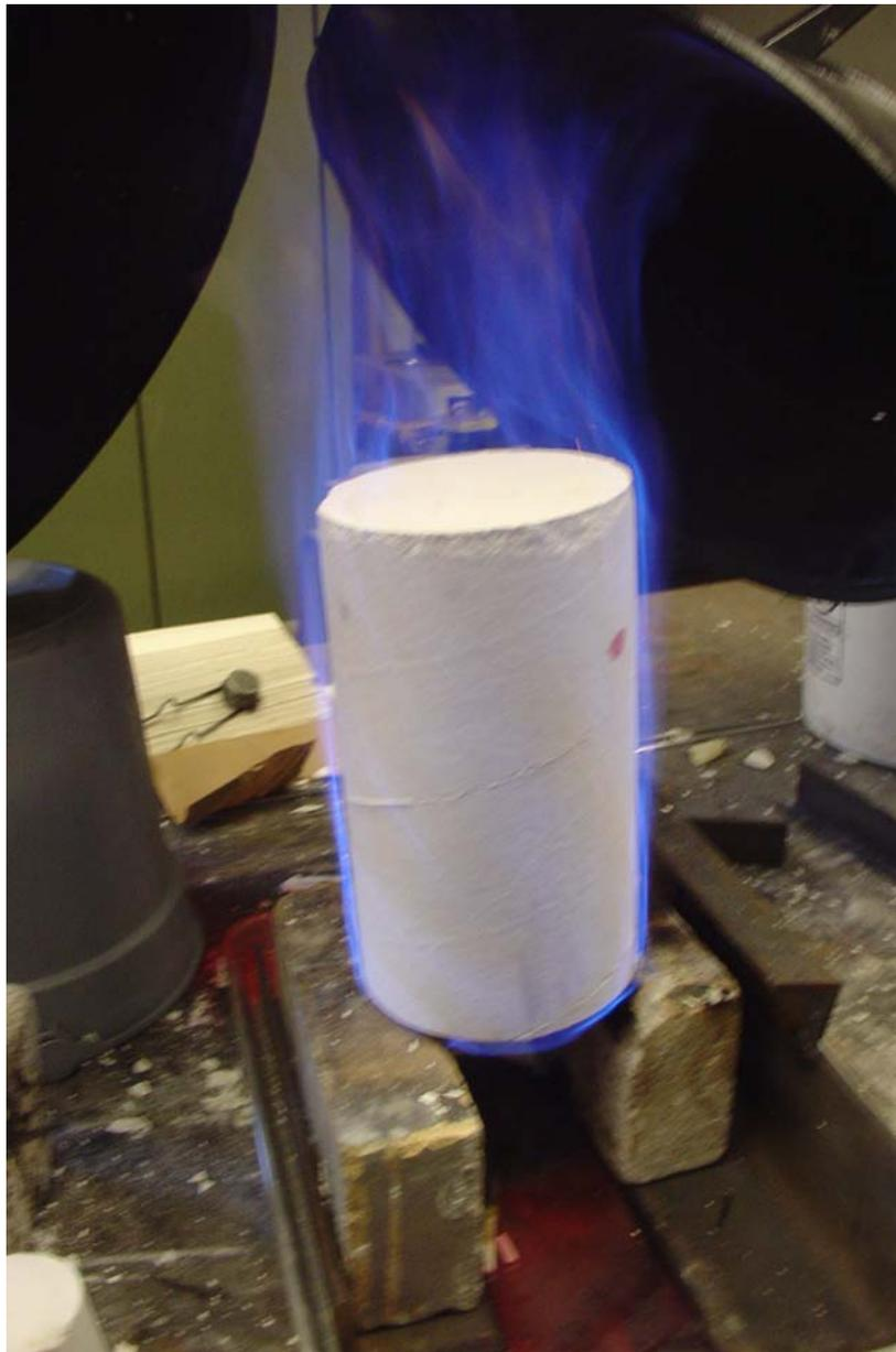
Burning ethanol-based binder to de-wax mold
