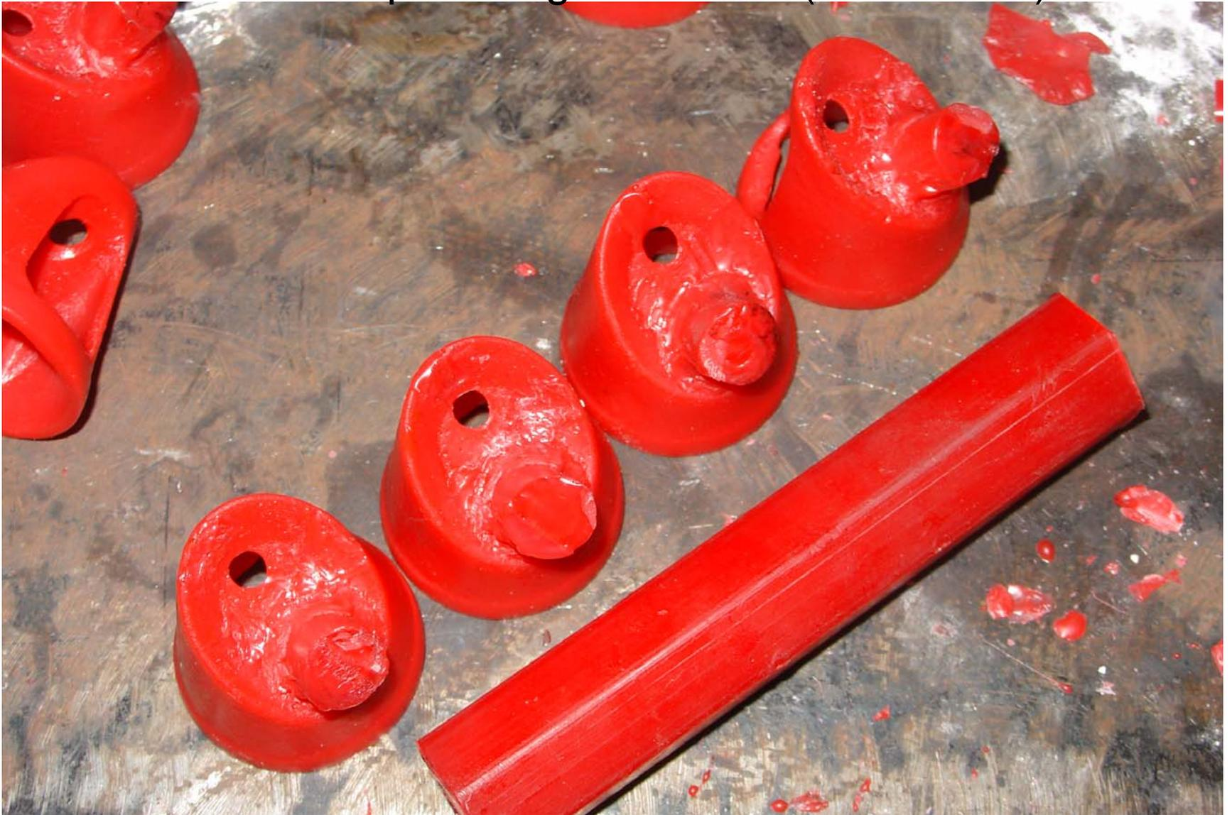
Multiple waxes created from a single rubber mold
