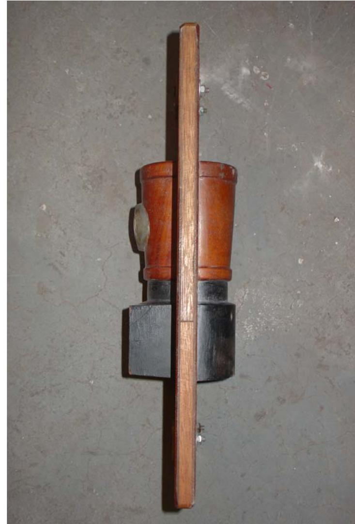
Above is a sand casting pattern. This is a model of what is cast
