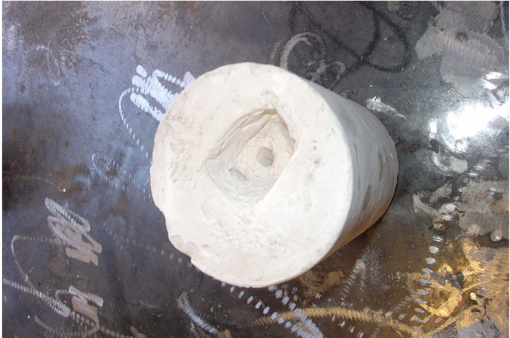
De-waxed ceramic mold ready for pouring
