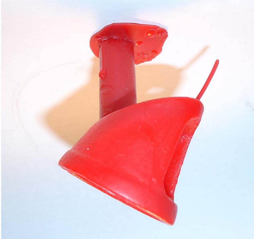
The most crucial part of lost-wax casting is producing a quality wax model. The metal you cast will be a very close replica of your original wax. Even fingerprint-level detail can be transferred from wax to metal. This wax is a wall-mount bottle opener.
