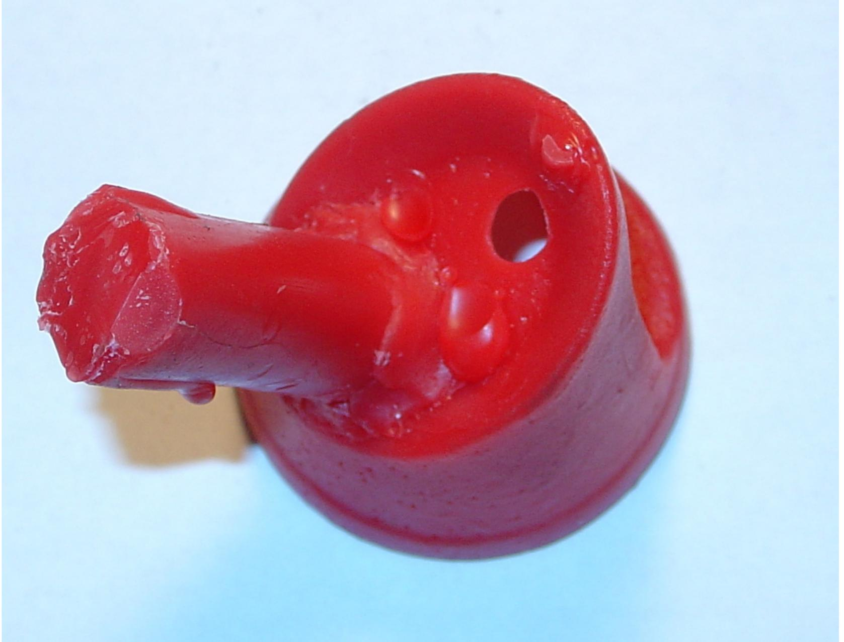
A finished wax, as removed from the rubber mold
