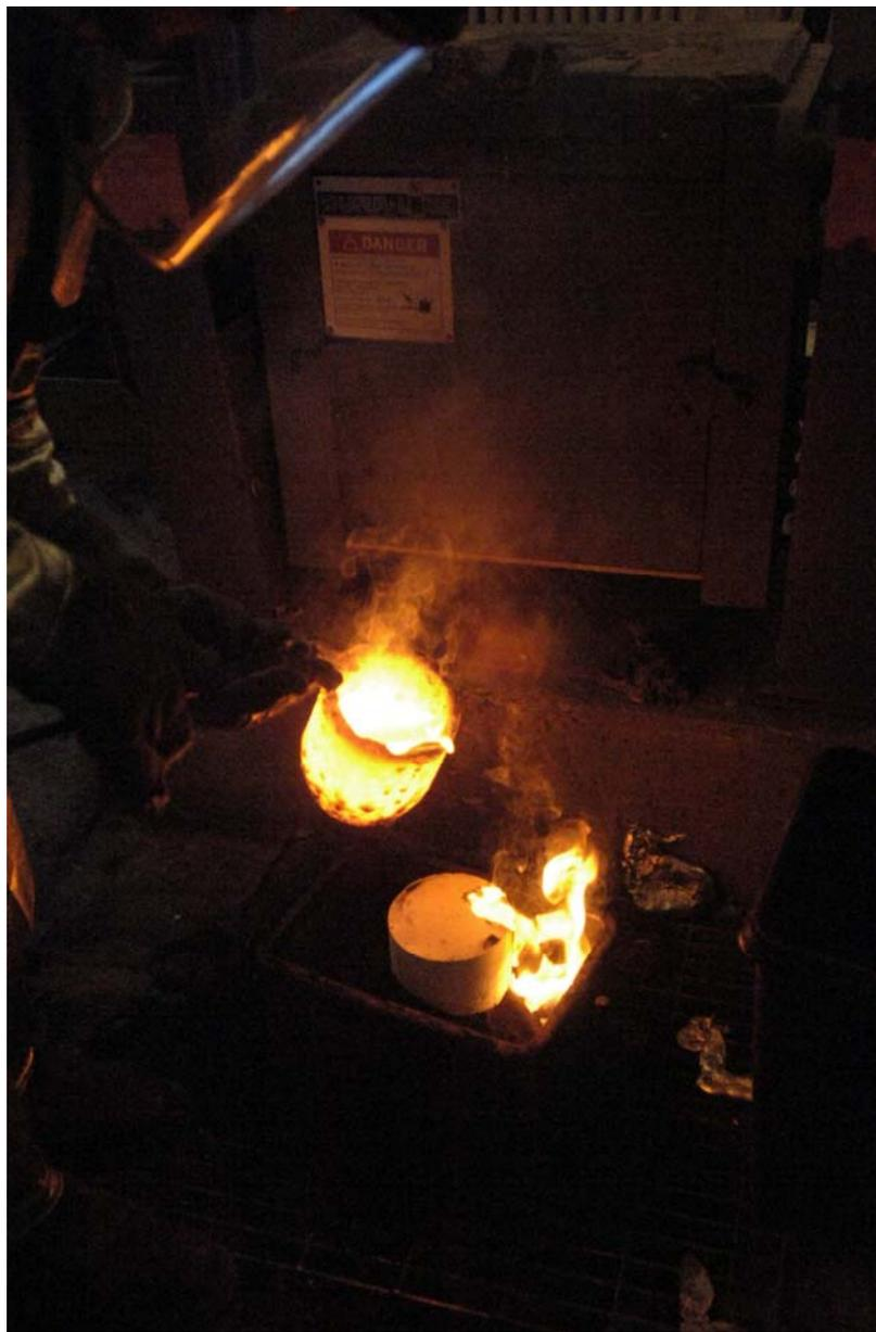
Pouring molten silicon bronze into a ceramic mold
