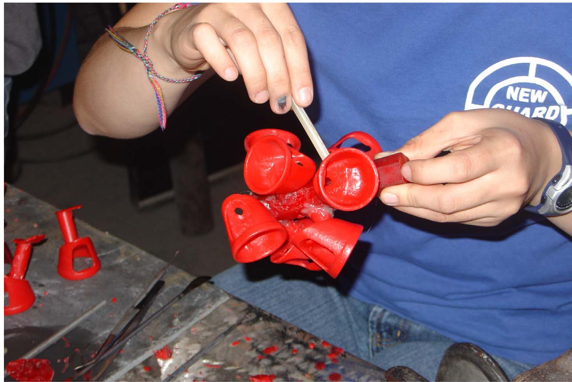
Attaching gated objects to central sprue to make wax "tree"
