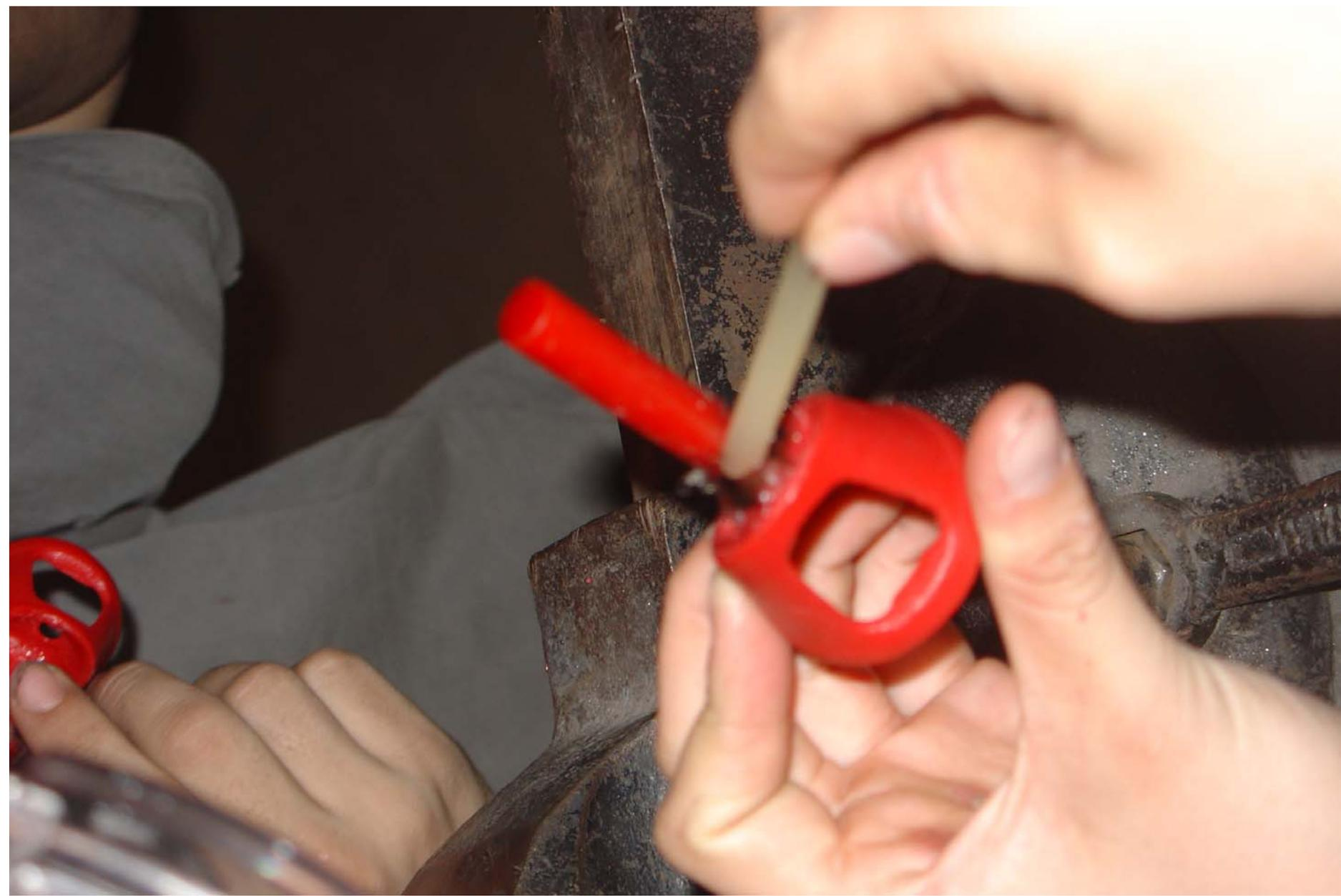
Attaching gates to wax objects using “sticky wax” as adhesive
