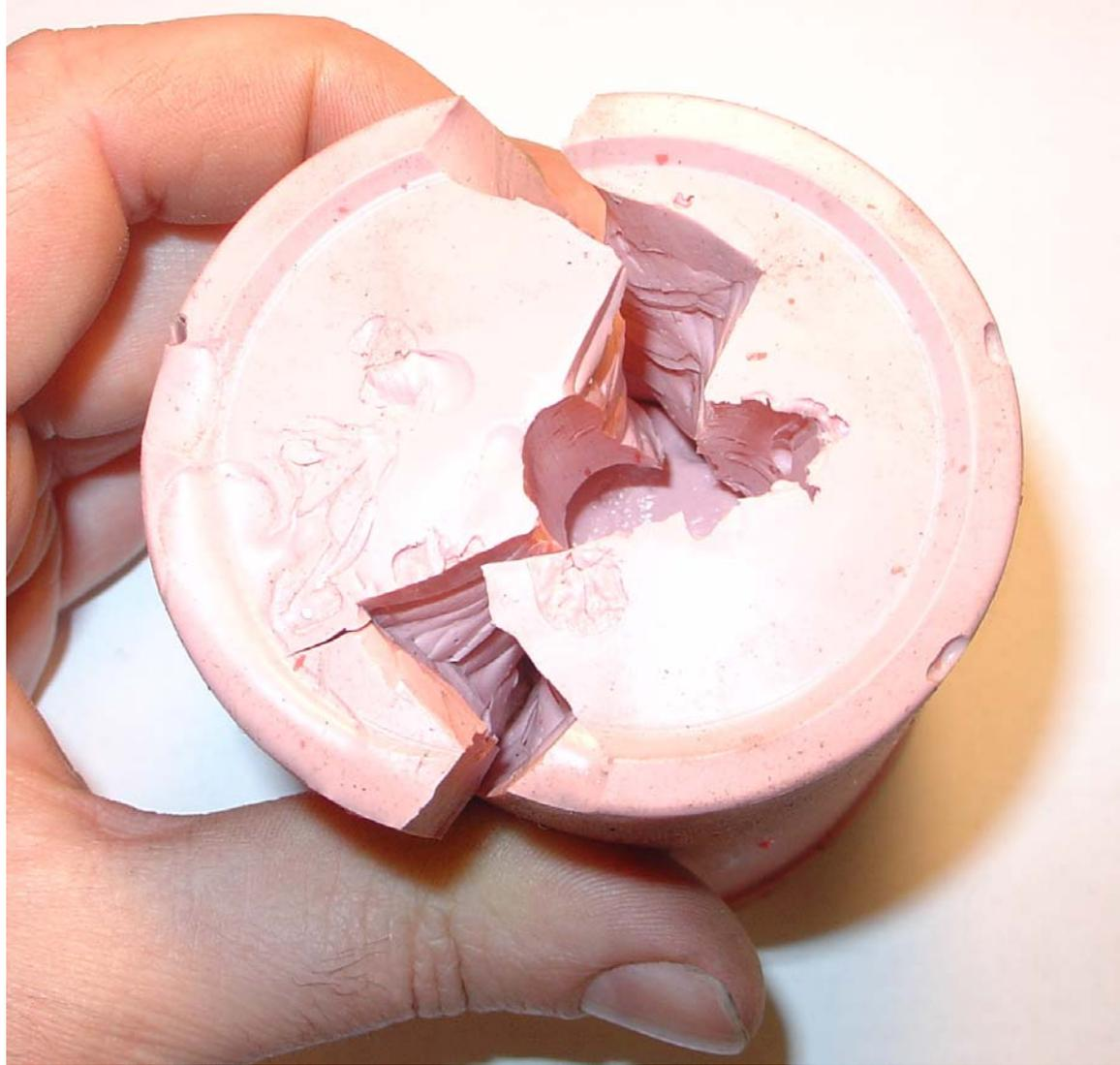
Here is a rubber mold made around the previous bottle opener. Once the rubber hardens, you remove the object and are left with a cavity that is an exact copy of the molded object. Molten wax is then poured into the cavity to produce wax copies.
