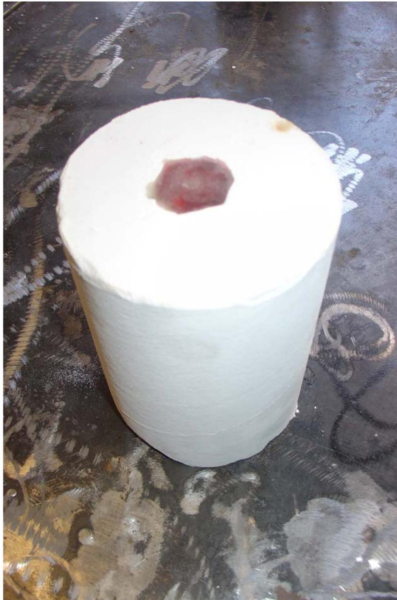
Finished mold with wax sprue evident
