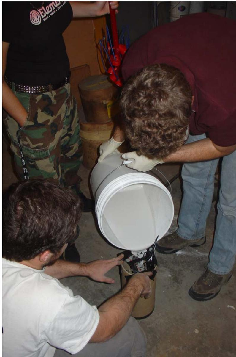
Pouring ceramic slurry over a wax tree, contained in a Carboard mailing tube
