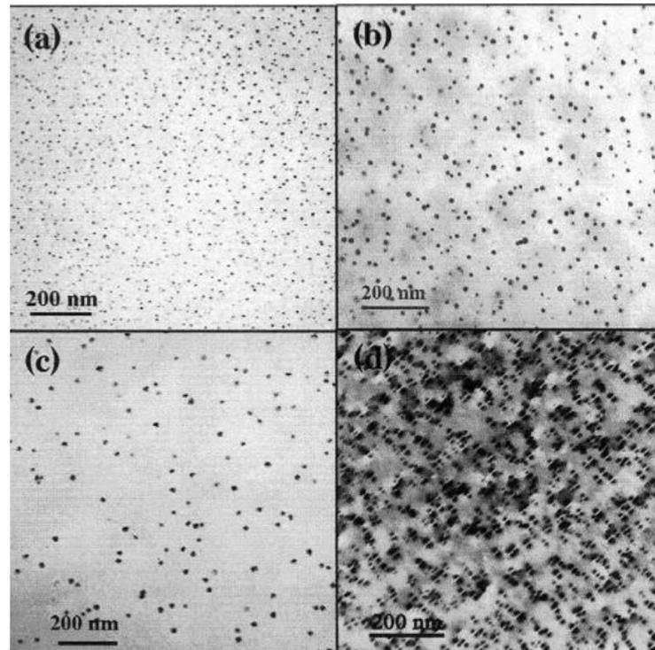
*Heat-treatable Al(Sc) transmission electron micrographs from D.N. Seidman et al. Acta Materialia 50 (2002) 4021-4035.*
