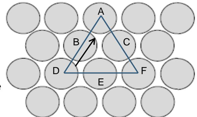
The FCC unit cell has a slip system consisting of the  $\{111\}$  plane and the  $\langle 110 \rangle$  directions.
