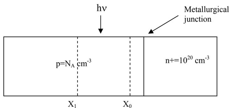
Note this is a n<sup>+</sup>-p junction. Without reverse bias, the depletion region on the p-side is labeled X<sub>0</sub>, whereas when a reverse bias V<sub>R</sub> is applied, it becomes X<sub>1</sub>. Light is entering as shown by the arrow.
