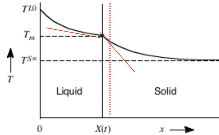
$$(J^L - J^S)_{x=X} \delta t = -K^L \left( \frac{\partial T^L}{\partial x} \right)_{x=X} \delta t + K^S \left( \frac{\partial T^S}{\partial x} \right)_{x=X} \delta t = \rho H_m \delta X$$
