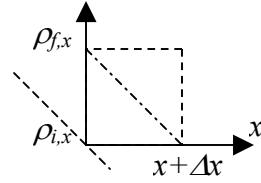
At time  $t = t_o$ , we know that the density at  $x = x$  is  $\rho_{f,x}$ , and we want to know the density at  $x = x + \Delta x$ . The slope of the density profile can also be written as  $\frac{\partial \rho}{\partial x} \approx \frac{\rho_{f,x+\Delta x} - \rho_{f,x}}{\Delta x}$ .
