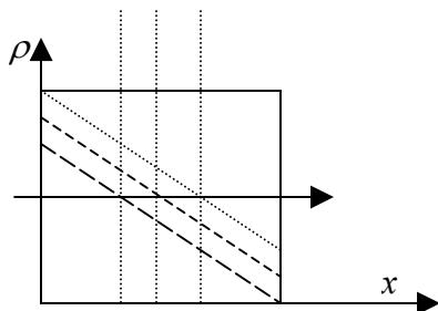
differential element increases with time, then the product  $u_x \frac{\partial \rho}{\partial x}$  must be negative. For fluid/body moving in a positive  $x$ -direction, the density gradient must be negative. Following the trajectory of the particle with time (denoted by the vertical lines), it is shown here that the density remains the same from the particle's frame of reference. Is this just a coincident?
