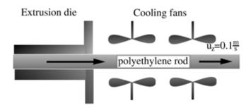
A cylindrical high-density polyethylene rod 0.02 m in diameter is exiting an extruder at a uniform rate of  $0.1 \frac{m}{\text{sec}}$  and a temperature of 160° C. It is cooled by fans to room temperature which is 40° C, with a heat transfer coefficient of  $130 \frac{W}{m^2 \cdot K}$ .
