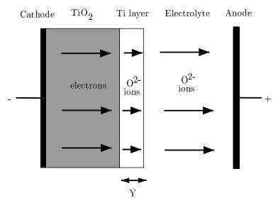
FFC-Cambridge process, shown in planar geometry for simplicity (the real process uses an approximately cylindrical geometry with the electrode at the center).
