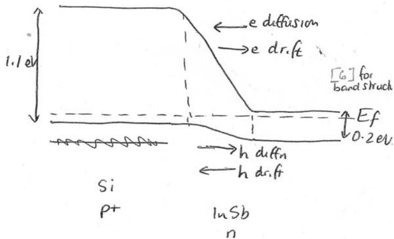
Electron currents and hole currents only in the depletion region. No net current.
