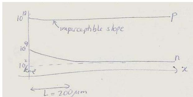
$$L = \sqrt{Dt} = \sqrt{40 \times 10^{-5}} = 2\sqrt{10^{-4}} \text{cm} \text{ or } 0.02 \text{cm} = 200 \mu\text{m}$$
