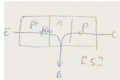
Large currents flow from E to B and from C to B. The current exits at B.
