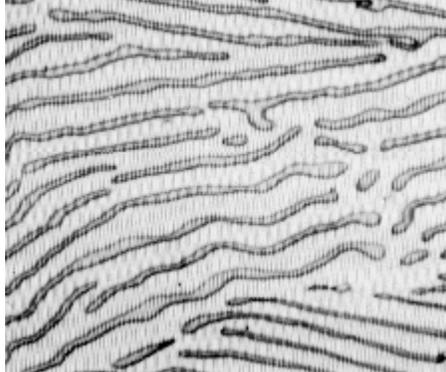
Martensite grains (gray) in austenite developed by rapid quenching.
