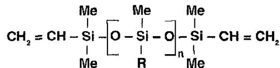
Curing via methylhydrogensiloxane with platinum catalyst:
