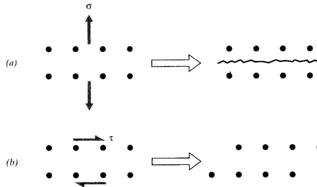
Figure 2: Cracking is caused by normal stresses (a), sliding is caused by shear stresses (b).
