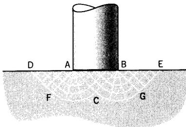
Figure 16: Slip-line construction for a flat indentation.
