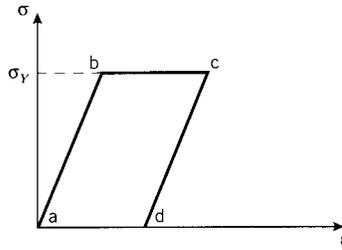
Figure 13: The elastic-perfectly plastic idealization of plastic deformation.
