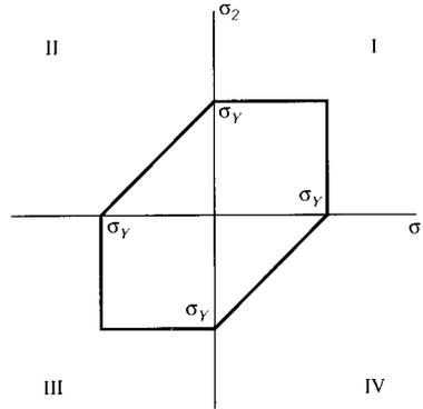
Figure 5: Yield locus for the maximum-shear stress criterion.
