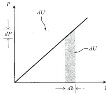
Figure 9: Increments of strain and complimentary strain energy.
