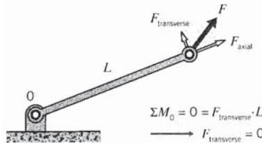
Figure 2: Pinned elements cannot support transverse loads.
