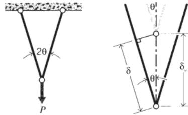
Figure 7: Two-element truss.
