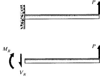
Figure 4: Wall reactions for the cantilevered beam.
