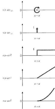
Figure 11: Singularity functions.
