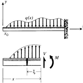
Figure 6: A distributed load and a free-body section.
