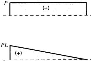
Figure 5: Alternative shear and bending moment diagrams for the cantilevered beam.
