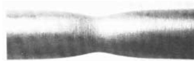
Figure 4: Necking in a tensile specimen.
