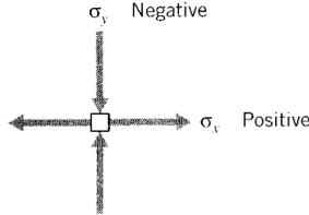
Figure 2: The sign convention for normal stresses.
