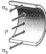
Figure 5: Hoop stresses in a cylindrical pressure vessel.
