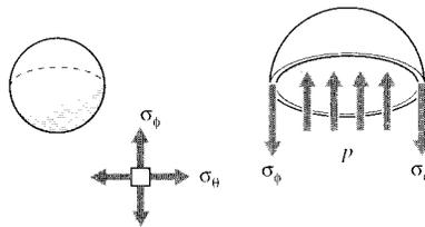
Figure 3: Wall stresses in a spherical pressure vessel.
