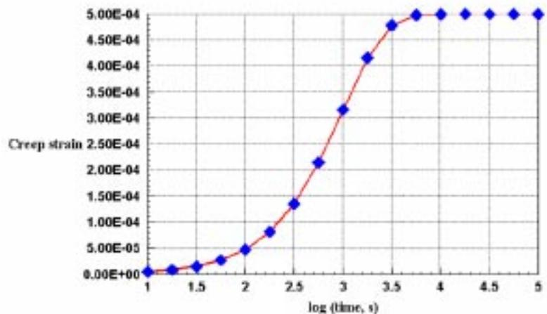
Figure 7: Creep strain history in model laminate.
