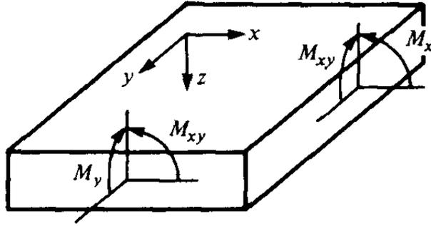
Figure 4: Applied moments in plate bending.
