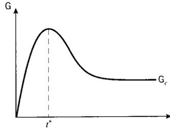
Figure 9: Effect of specimen thickness on toughness.
