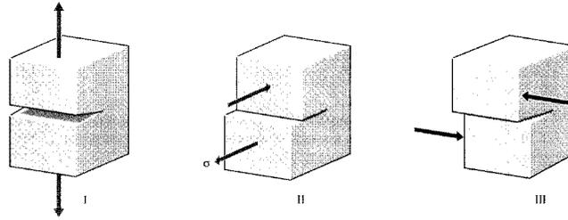
Figure 6: Fracture modes.
