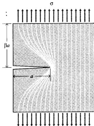
Figure 1: Idealization of unloaded region near crack flanks.
