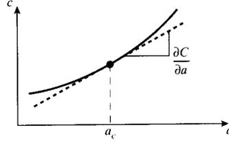
Figure 4: Compliance as a function of crack length.
