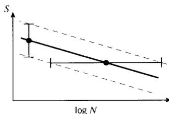
Figure 5: Variability in fatigue lifetimes and fracture strengths.
