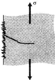
Figure 1: Intrusion-extrusion model of fatigue crack initiation.
