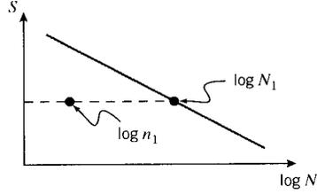
Figure 8: The concept of fractional lifetime.
