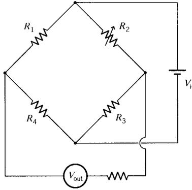
Figure 2: Wheatstone bridge circuit for strain gages.
