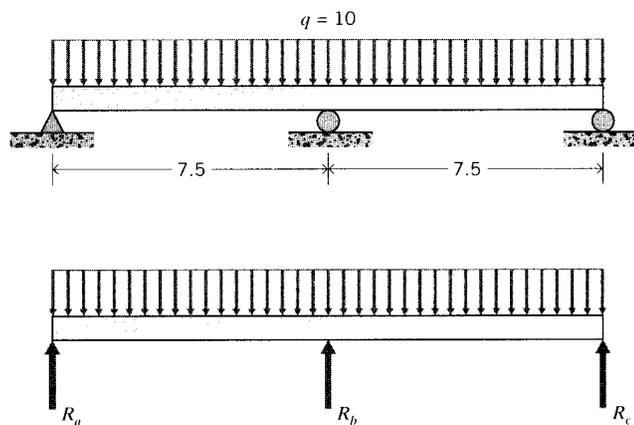
Figure 2: Uniformly loaded beam resting on three supports.
