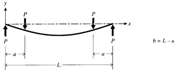
Figure 7: Four-point bending.
