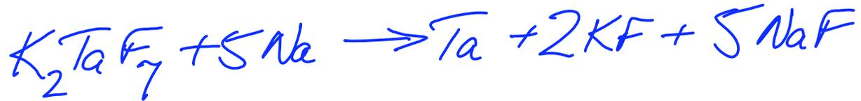
(b) A reactor is charged with 222 kg of  $K_2TaF_7$  and 6.66 kg of Na, and the reaction is allowed to go to completion. Calculate how much tantalum is produced. Express your answer in kg.
