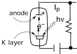
$I_p$ , the photocurrent, is proportional to the intensity of incident radiation, i.e. the number of incident photons capable of generating a photoelectron.
