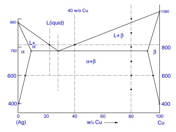
(b) Determine the liquidus temperature for a 60 wt.% Ag - 40 wt.% Cu alloy.
