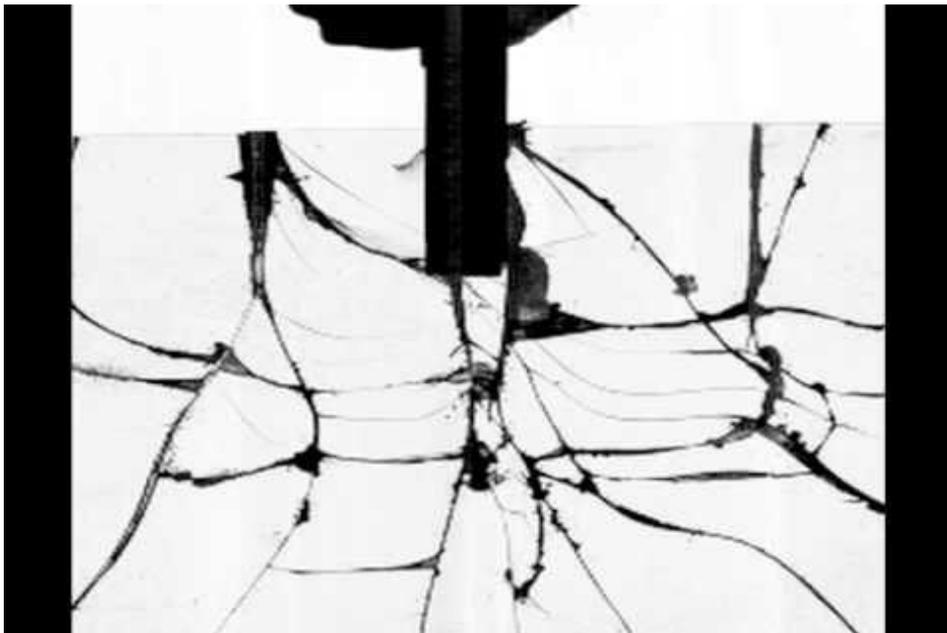
Glass cracking at 231,000 fps
