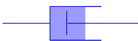
A blue square with a vertical line through its center, representing a dashpot, connected to horizontal lines on both sides.
