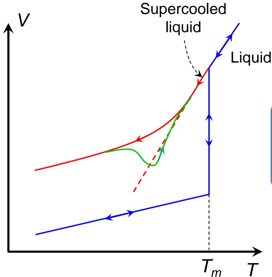
The heating curve never retraces the cooling curve during glass transition due to structural relaxation
