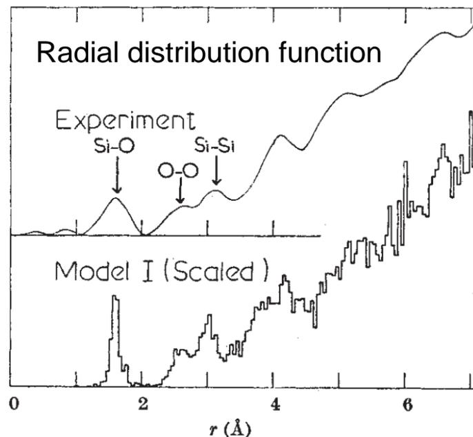
Excellent agreement between XRD and ball-and-stick model constructed according to the random network model
