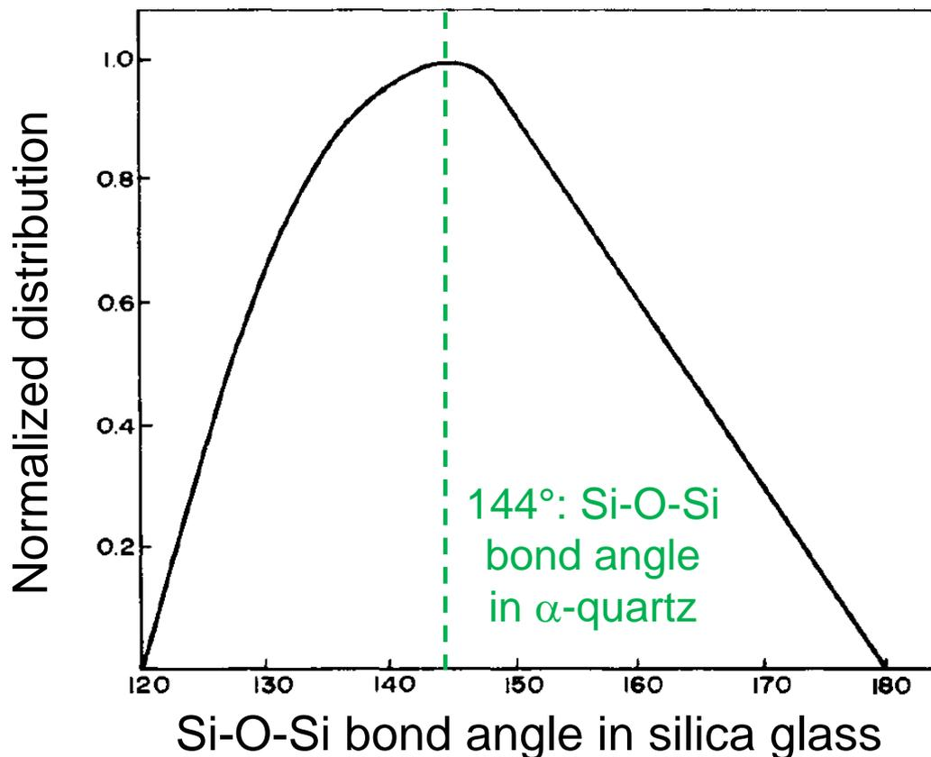
Si-O-Si bond-bending constraint is relaxed at the forming temperature of silica glass
