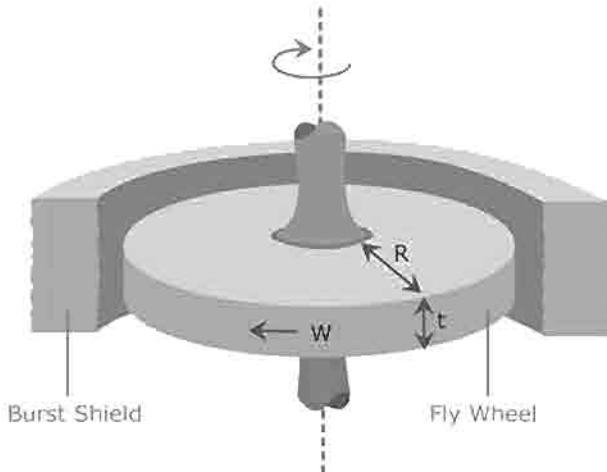
$$\text{Kinetic energy: } U = \frac{1}{2} I \omega^2 = \frac{1}{2} \left( \frac{\pi}{2} \rho R^4 t \right) \omega^2$$
