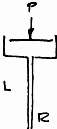
$$0 = -\frac{\partial P}{\partial z} + \frac{\mu}{r} \frac{\partial}{\partial r} \left( r \frac{\partial u_z}{\partial r} \right)$$
