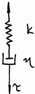
$$\dot{\gamma} = \dot{\gamma}_s + \dot{\gamma}_d = \frac{\dot{\epsilon}}{k} + \frac{\gamma}{\eta}$$
